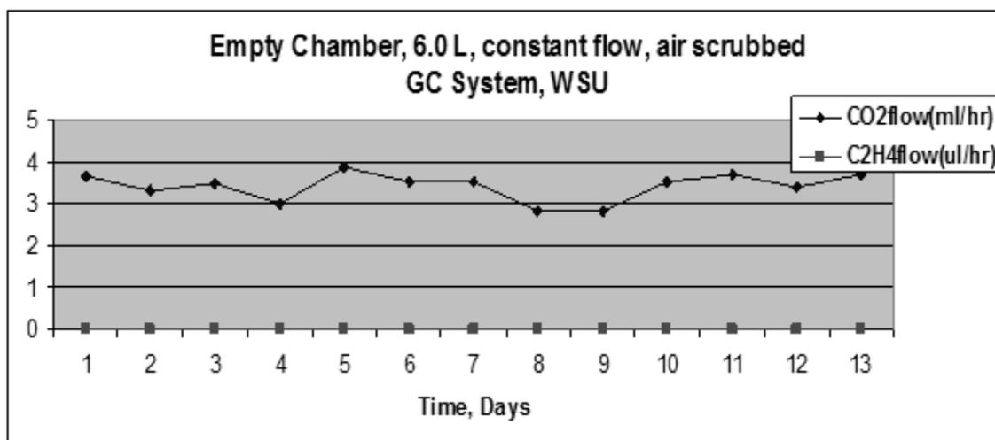
**Figure 4.** Blanking calibration in GC based system (top) and CID-900 instrument (bottom) with 400 mL/min dynamic flow through sample chamber. Note continuously lower ethylene values than GC-based technology.
