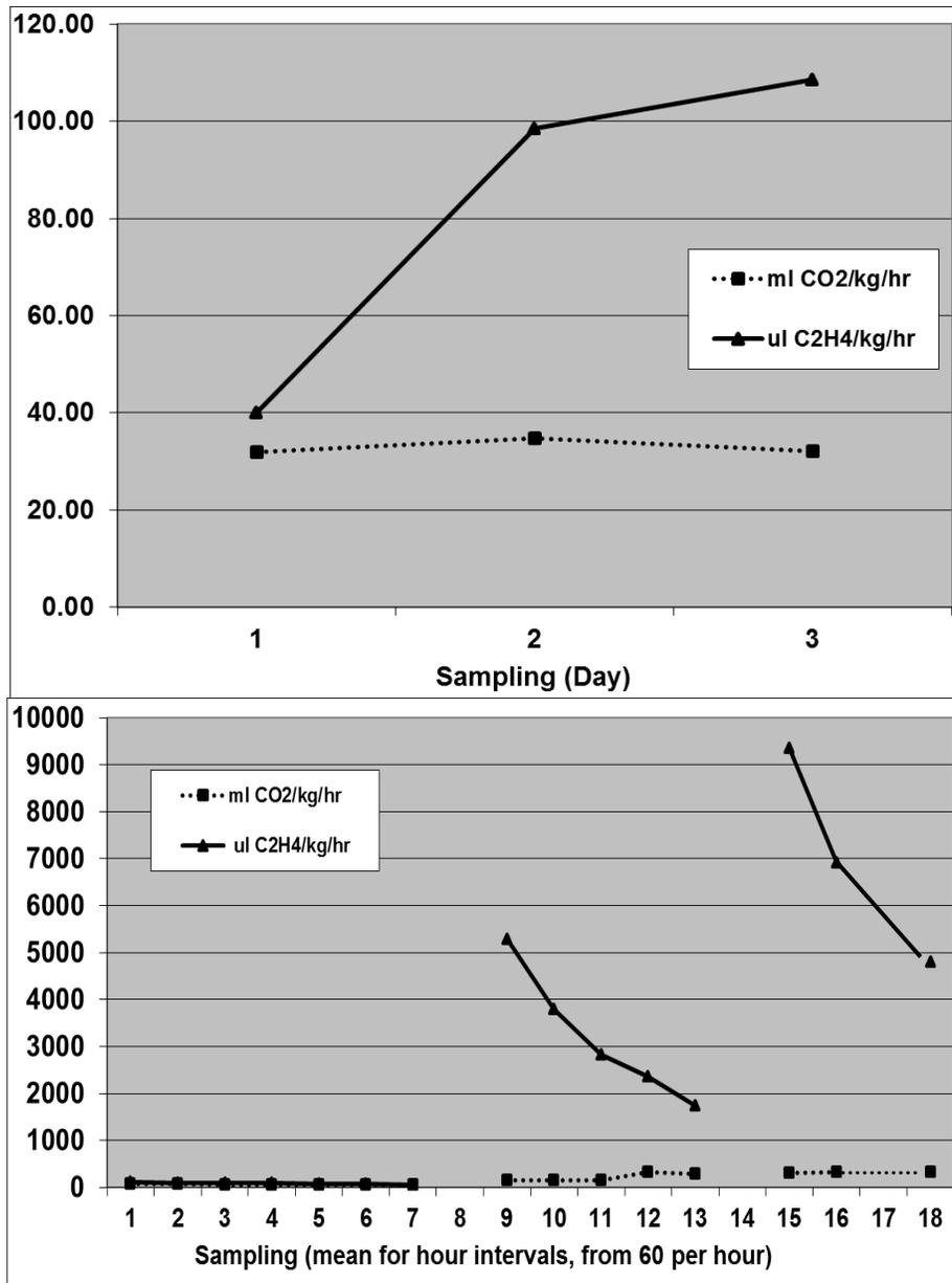
**Figure 5:** Comparison of existing gas-chromatography based respiration monitoring (Top) and CID-900 real-time ethylene and carbon dioxide monitoring instrument (Bottom). A dynamic flow was established in the headspace of the chamber measured by the CID-900 instrument between sampling events 7 and 9 at 400 mL/min flow rate. Note enhanced resolution in data from CID-900 instrument in comparison.
