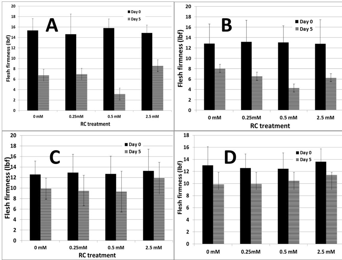
**Figure 3.** Flesh firmness reduction in SmartFresh-treated, RC2 exposed Anjou fruit from the 2013 season. (A) and (B) represent firmness reduction in Bartlett and Anjou (respectively) after 24 hour RC2 exposure. (C) and (D) represent firmness reduction in Bartlett and Anjou (respectively) for 12 hour RC2 exposure. Error bars represent standard deviation from the mean. The 12 hour exposure prevents significant losses in flesh firmness associated with ripening.
